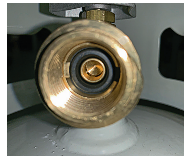
This is a 20-pound cylinder with an OPD valve and face seal that is in good condition.
